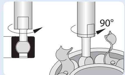
Insert the second adapter into prepared area diametrically opposed.
