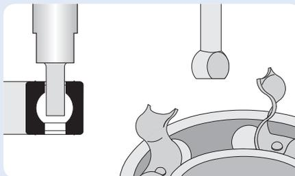
Insert appropriate bearing adapter and rotate it 90° ensuring positive grip within the bearing race.
