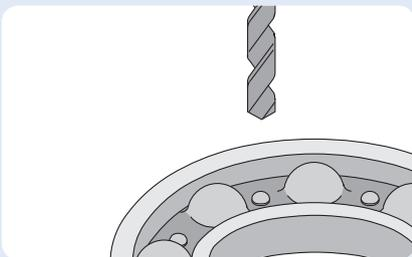
Remove seal and open selected section of ball cage. Clean the swarf out.
