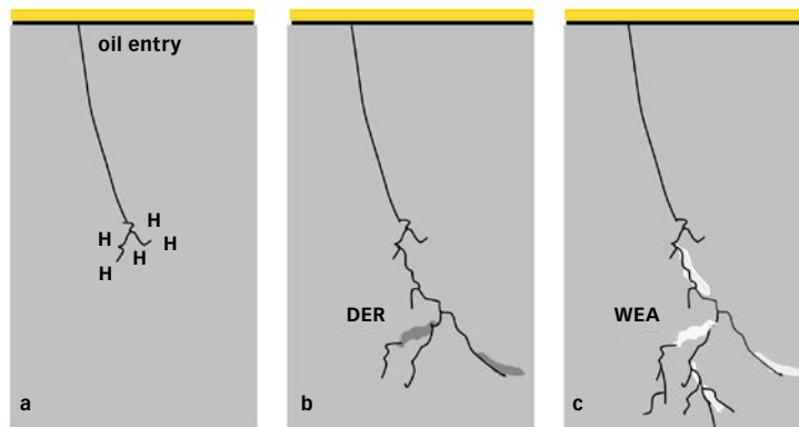
Fig. 12 (continuation of fig. 8): a) After penetration, oil and additives react in the crack flanks locally producing hydrogen, b) and c) the hydrogen transforms locally the microstructure close to the crack system into white etching cracks WEC (from dark etching regions, DER, to white etching areas, WEA) 6, 7, 16 .
