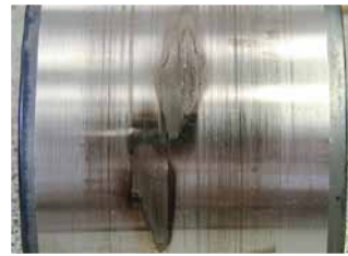
b) sliding damage/smearing;
