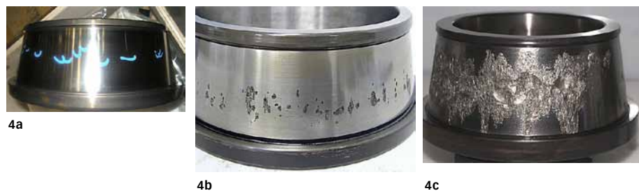
Fig. 4: Failure appearance: a) straight cracks, b) straight cracks and small spalls, and c) spalls.
